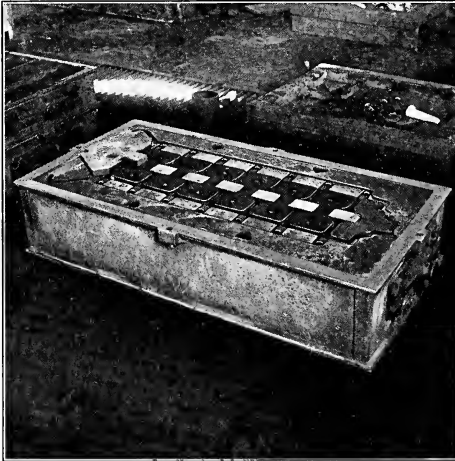
Fig. 62. Drag Half of Mould with Cores Set.
